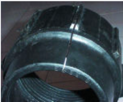
Failed nut with longitudinal split
