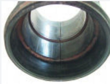
Failed body with longitudinal split
